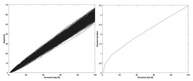
The noise present on the ramp reference voltage is itself directly translated to output ADC digital number noise, which degrades image quality and is highly visible under low light illumination in the case of a CMOS image sensor. Depending on the ramp generator type the current noise on the ramp reference could undergo integration and present itself with high absolute deviations in long integration time scenarios.
