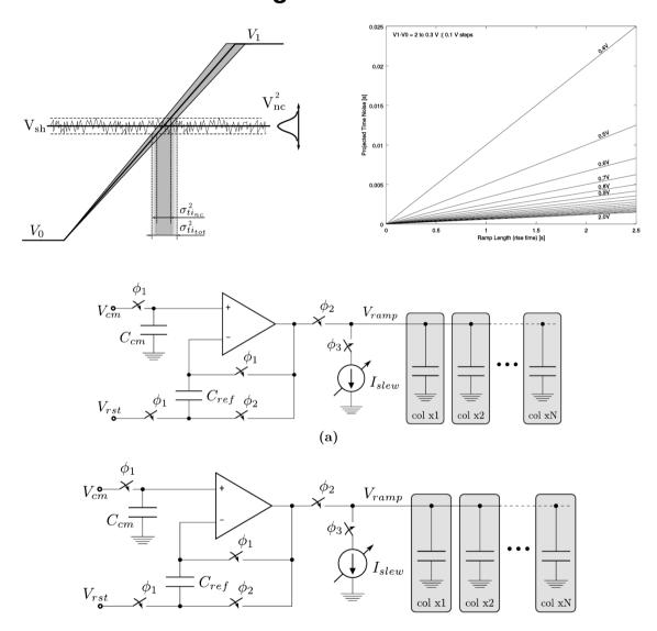
The Single-Slope, often known as ramp ADC is the most common type of column-parallel ADC used in CMOS image sensors and high-precision instrumentation measurement analog front ends. It offers favorability to CMOS process node scaling and excellent area requirement. However, unlike other types of ADCs, the ramp ADC needs a source of linear voltage generation which is
